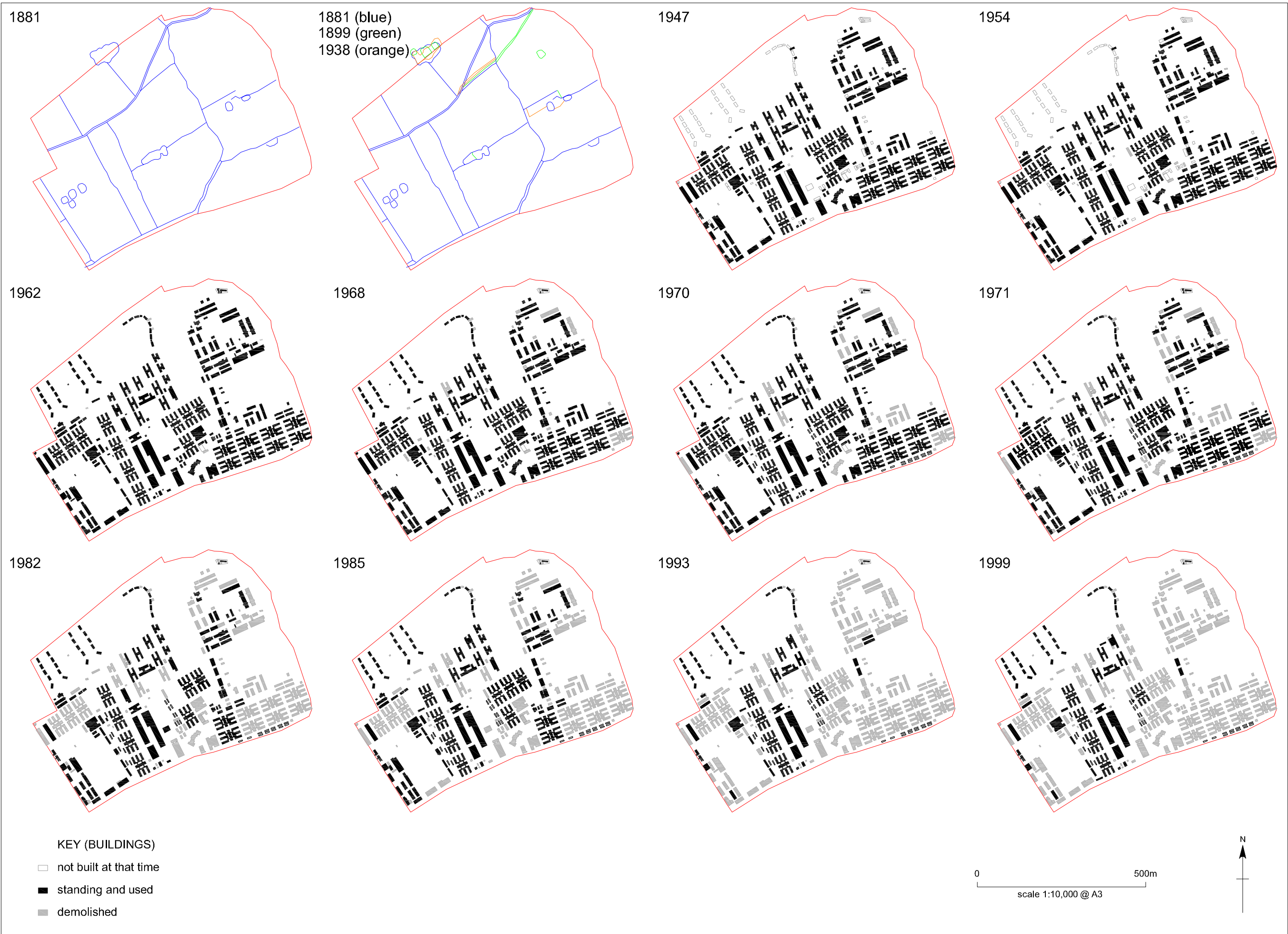
Figure 3 Saighton Camp, Chester: development of camp based on Ordnance Survey mapping and aerial photographs
